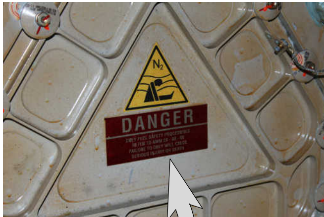
Nitrogen enriched air flooded center tank
