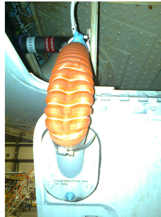
Oxygen enriched air outlet (attached to 3" HP GRD connector panel)
