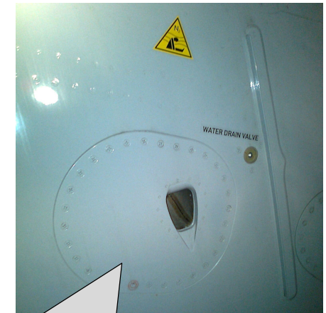
Nitrogen enriched air out of NACA inlet
